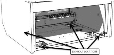
Once all the bolts are removed, slide the unit off the back of the shipping pallet, and tilt it so the rear corner touches the ground. Then have someone move pallet out from under the case and gently tilt the case forward until it touches the floor. Shelves, doors, and front glass may be removed from the unit to reduce overall weight.
